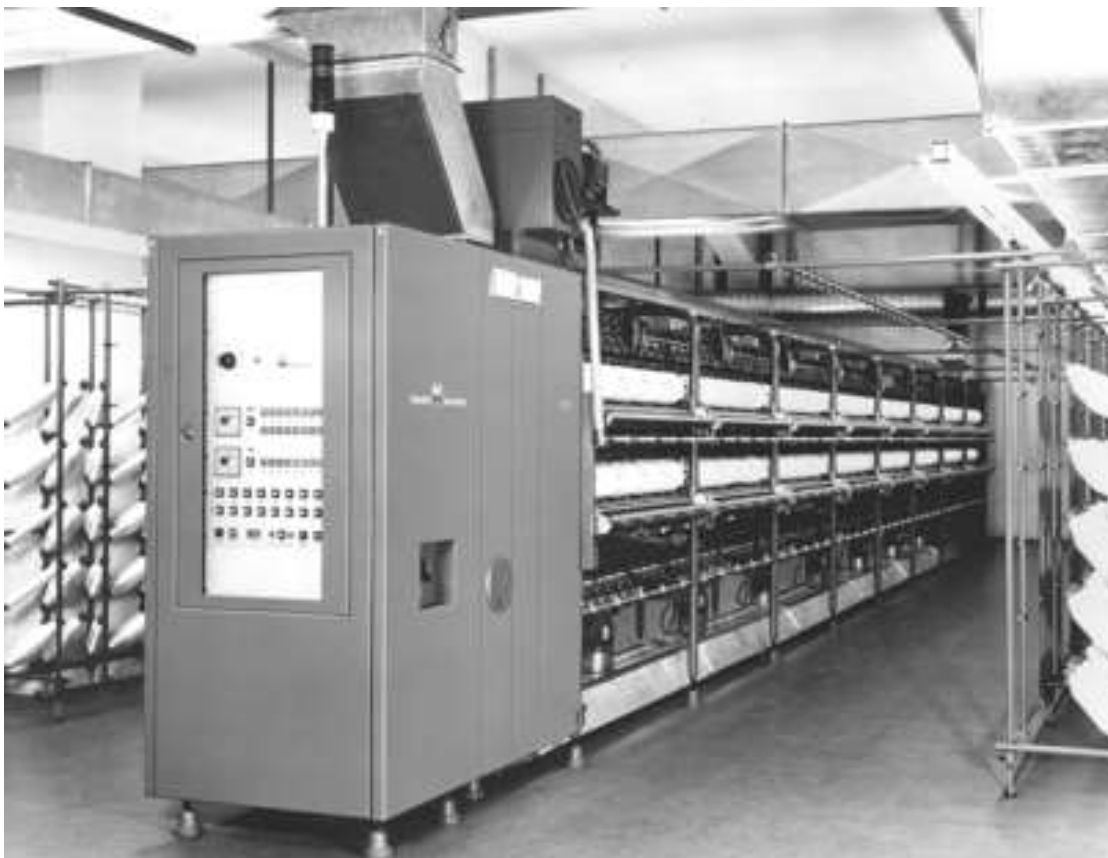
Heberlein false-twisting machine manufactured around 1950
